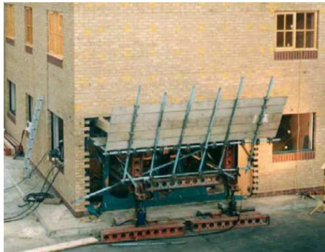
Figure 4.11: Disproportionate collapse test (Mettem et al., 1998)
