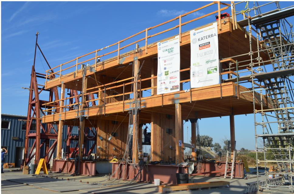
Figure 2.1: Two-story structure tested during the summer 2017 at the UC San Diego outdoor shake-table
